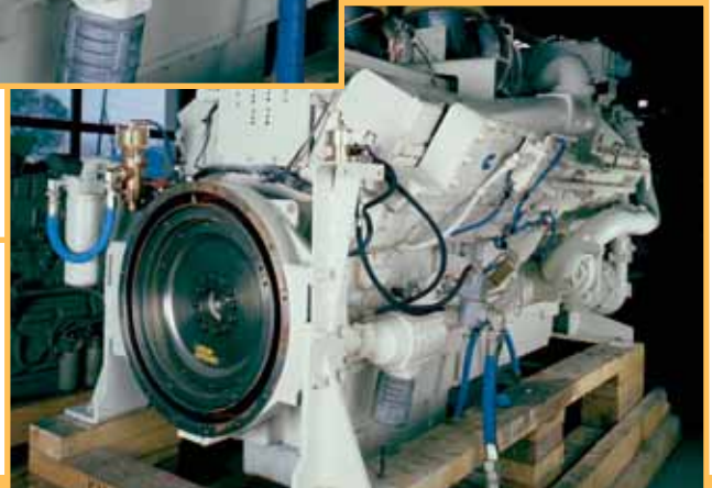
The SS815GB03R31 starter is shown mounted on a Cummins KTA50-M2 piped with the IR SRV150 Relay Valve.
