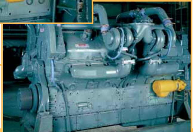
An ST650BP03R31 starter is shown mounted on a Detroit Diesel 12V-149R.
