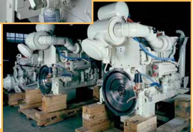
The 150BMGE21RH-6 starters are shown mounted on a Cummins KTA14-M3 and KTA19-M4I.
