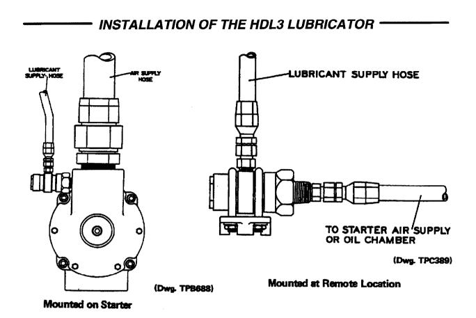
The HDL3 Lubricator is self-priming and may be installed directly on the Starter or remotely located. Although the Lubricator is capable of drawing lubricant from a source 4 ft (1.2 m) lower than the point of installation, we recommend installing the Lubricator as close as possible to the oil source.
