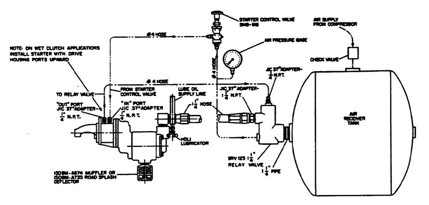
NOTE: USE I-R SMB-441 SEALANT ON ALL PIPE CONNECTIONS.
