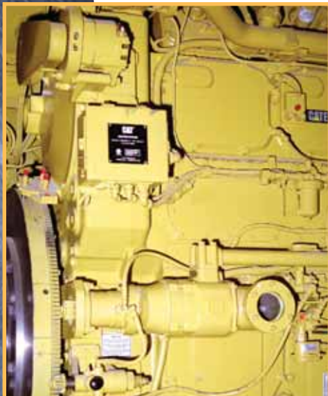
The ST999BP03R31 starter is ready for use on a Cat 3608 engine.
