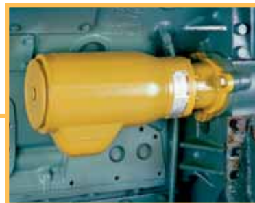
An ST650BP03R31 starter is shown mounted on a Detroit Diesel 12V-149R.
