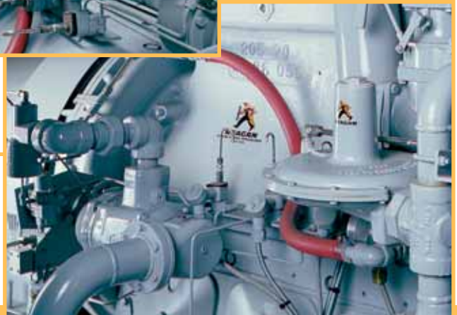
The ST799GCDP03R31 starter is piped for use with gas on a Waukesha F3521GU used for power generation.
