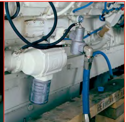
The SS815GB03R31 starter is shown mounted on a Cummins KTA50-M2 piped with the IR SRV150 Relay Valve.
