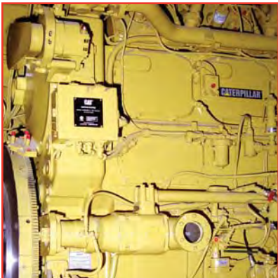
The ST999BP03R31 starter is ready for use on a Cat 3608 engine.
