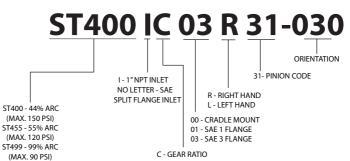
When ordering a Starter, refer to table below for correct pinion data.
