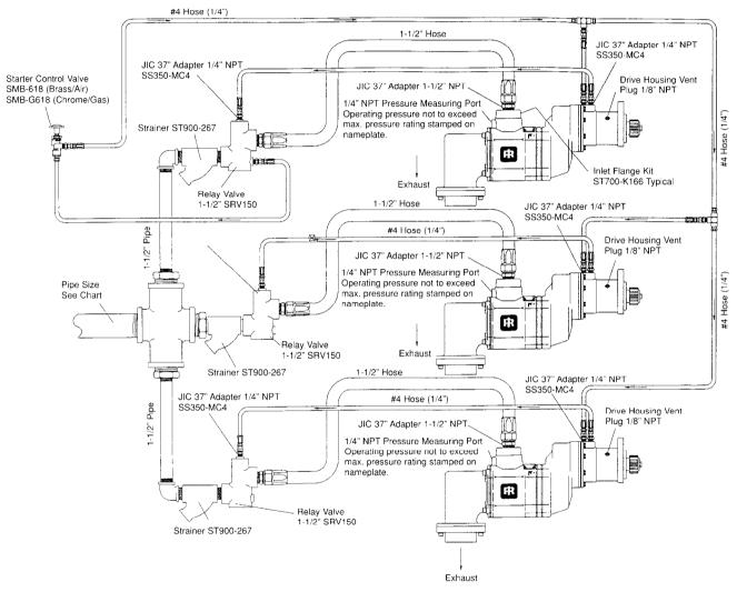
Supply must be adequate to maintain desired operating pressure at the starters with starters running. (Not to exceed max. pressure shown on starter nameplate.)
