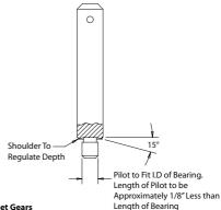
**Needle Bearing Tool For Planet Gears**
